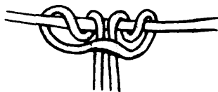
The Prusik knot is used to tie one rope around another. One rope will slide along the other if there is no tension, and it will hold if tension is applied. This knot should be tied off with a bowline.
